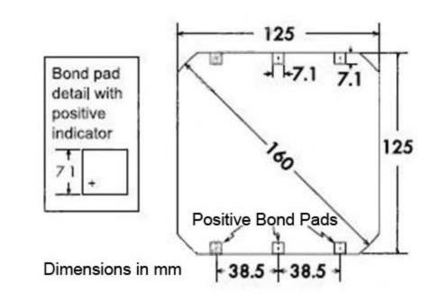
Bond pad area dimensions are 7.1mm x 7.1mm Positive pole bond pad side has"+" indicator on leftmost and rightmost bond pads.
